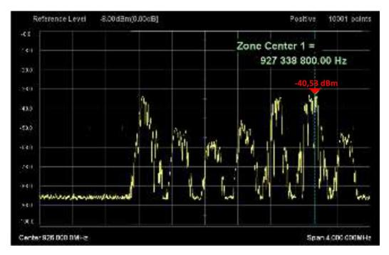
It is suspected that such RF noise could be generated by multiple Wi-Sun smart meters in very close proximity with the Sigfox device.
