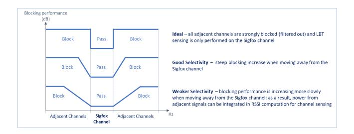
This **RSSI Selectivity or Blocking parameter** is fully dependent on the selected radio transceiver and device makers shall understand that the performance can widely vary from one provider to another.
