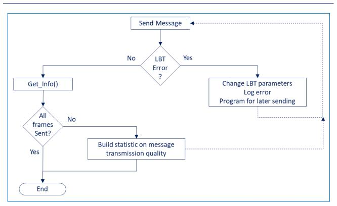
In the early phase of the deployment, during field tests/pilot, it is important to monitor the LBT mechanism both on device and backend side to build a learning database and tune the LBT mechanism to best suit the RF environment. This may require deploying a significant number of devices for a significant period as environmental parameters can widely change depending on location and overtime.
