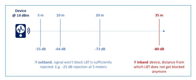
This chart is very theoretical: it assumes that other devices (transmitting in Sigfox or adjacent channels) can be localized. When deploying in dense urban area, a spectrum analyser could be used to assess the power of interferers in Sigfox channel as well as in adjacent channels.
