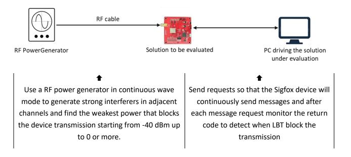
Doing such test will enable to build a table like the one below with for each adjacent frequency the value of the CW signal that will block the LBT:
